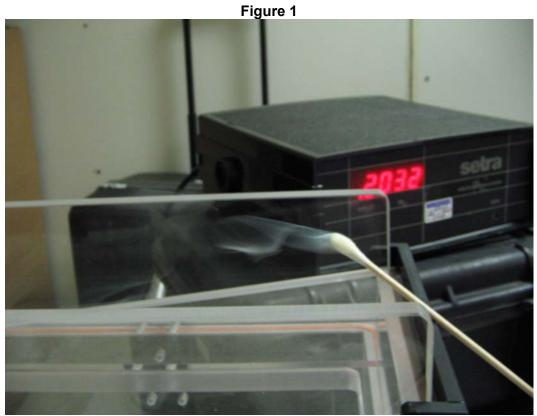
Elevation of 7-Liter Chamber Showing acceptable airflow capture at 0.20"wg vacuum. Airflow capture improves for all values of vacuum greater than 0.20"wc.
