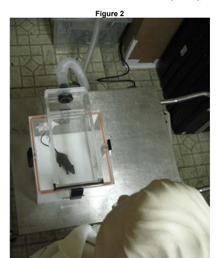
Tracer Gas Test Geometry (~14" viewing distance to top of 'Chamber; Simulated Rodent)
